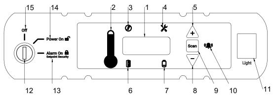
Figure 11. Refrigerator Control Panel
