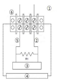
Figure 14. Temperature Transmitter
