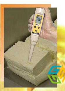
pH is one of the key parameters measured in food processing. The Eutech waterproof pH Spear with tough, spear tip open pore sensor is a rugged, user-friendly tester ideal for direct measurement of solid or semi-solid samples such as chéese, meats, fruits, bread and other similar samples.
