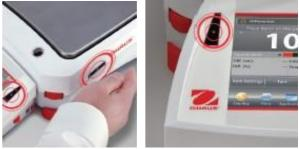
The sensors can be set up to provide automated operation of the draftshield side doors and can be programmed to automatically open the opposite side door to support efficient and logical sample placement with your free hand
